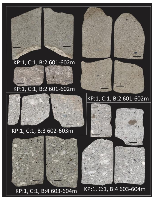
Figure 2. Scan images of vitro crystal tuff from the Kecerovské Pekľaň-1 well, core 1, boxes 2–4, depth interval 601–604 m. Box B:2 (601–602 m) – Tuffite. Appearance: Generally greyish, fine-grained, massive texture. Clast content: Sparse, small lithic and crystal fragments scattered within a dominant fine-ash matrix. Matrix: Predominantly altered volcanic ash with some detrital material, giving it a hybrid (volcaniclastic–sedimentary) character. Interpretation: Rock corresponds to tuffite – volcaniclastic material mixed with significant proportion of sedimentary particles, relatively poor in visible glass shards but occasionally includes large pumice fragments. Box B:3 (602–603 m) – Tuff (transition to tuffite). Appearance: Light grey to mottled texture with noticeable darker lithic fragments. Clast content: Abundant crystal and lithic fragments (plagioclase, quartz, volcanic lithics) are embedded in finer matrix. Some elongated pumice shards appear to be preserved. Matrix: Ash-sized material dominates, less massive than B:2, suggesting more direct pyroclastic input. Interpretation: Likely fine-grained tuff, possibly transitional toward tuffite, due to sediment admixture but with clear pyroclastic shard content. Box B:4 (603–604 m) – Vitro crystal tuff. Appearance: Light grey with conspicuous white elongated pumice fragments and darker lithic clasts. Clast content: High proportion of crystal fragments (feldspar, quartz) and lithics, set in an ash matrix. Pumice clasts show elongation and flattening, indicating compaction. Texture: More heterogeneous compared to B:2 and B:3.
